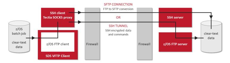
The Tectia SOCKS proxy server intercepts FTP traffic executed by the z/OS FTP client and sends FTP traffic via an encrypted tunnel or converts FTP to SFTP protocol.
